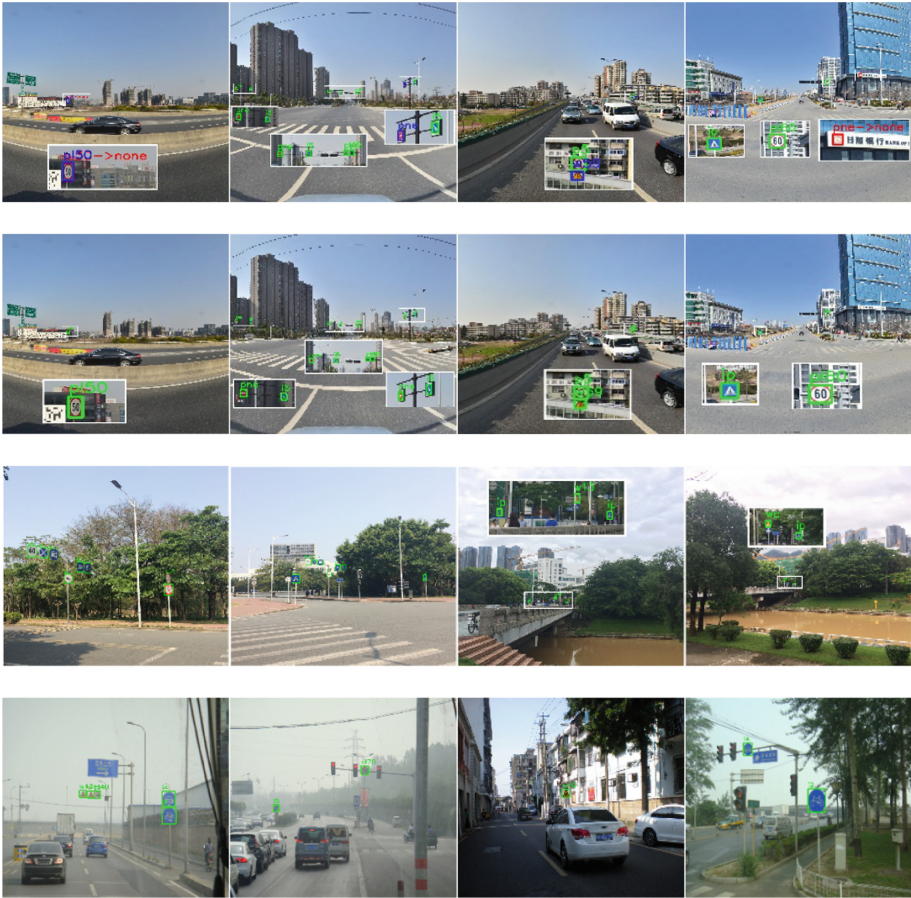
Fig. 9. The detection results on TT100K and the CTSD. The first row shows the detection results of Zhu et al. [1] on TT100K. The second row shows the detection results of our model on TT100K. The third row shows the detection results for our collected images. The fourth row shows the detection results of our model on the CTSD. The green, red and blue rectangles denote true positives, false positives and false negatives, respectively. (Color figure online)
