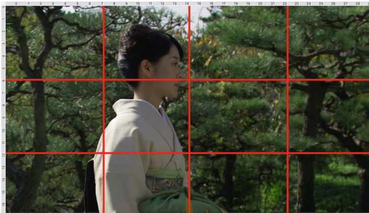
Fig. 2. Example of partitioning a frame into 12 tiles (Kimono sequence).
