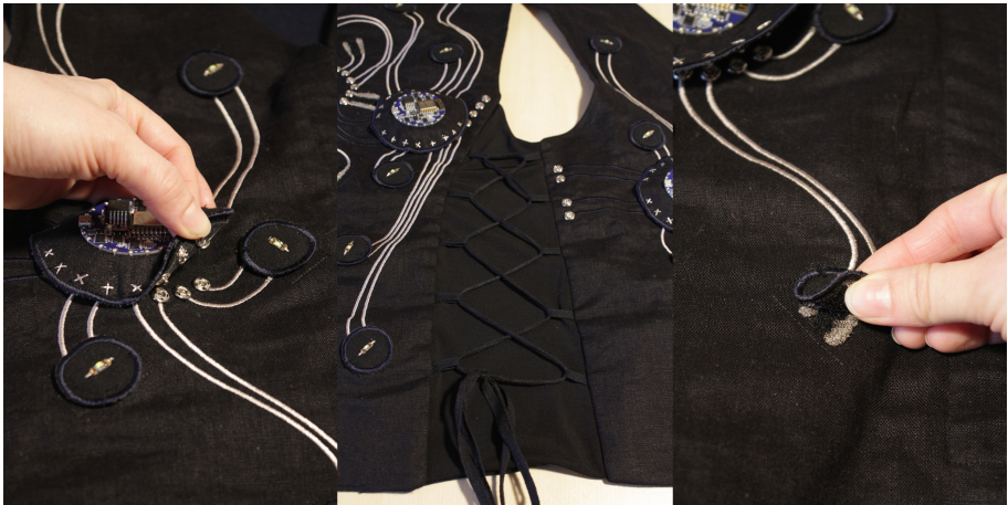
Fig. 4. (From left to right) Control boards are attached with metallic snap-on buttons. The fit of the vests can be adjusted by cinching down slack in the fit. Motors and LEDs are attached with conductive hook-and-loop tape. The small circular patches pictured here are LEDs, which coincide in position with the ERM motors that are on the opposite side of the garment (close to the wearer's body).
