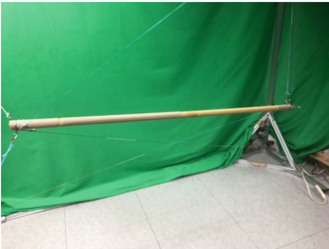
Fig. 6. An end effector used in rod tracking task.
