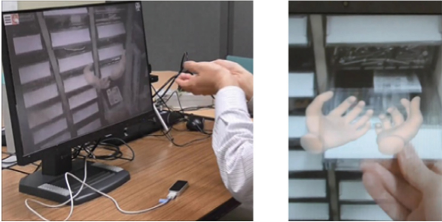
Fig. 3. Setup of the expert site (left), an image superimposed on the remote workers' eye-sight (right).
