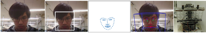
Fig. 6. Head-down detection for ARM-COMS control
