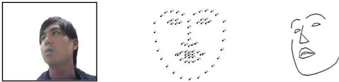
Fig. 4. Image-based processing to determine the face orientation
