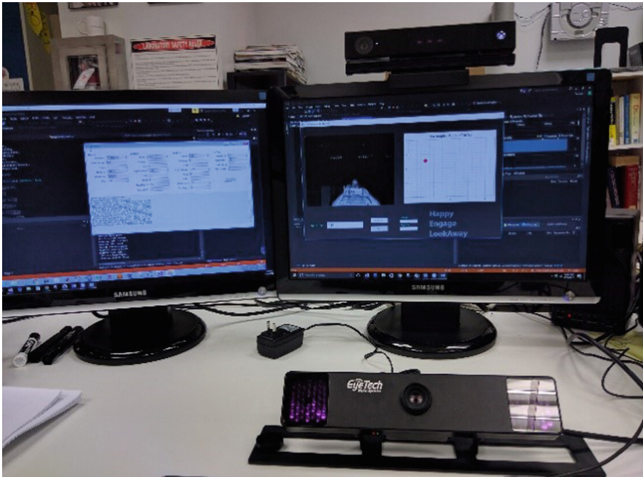
Fig. 1. An entire system including Kinect V2 (on top of the screen) and TM3 (in front of the computer)
