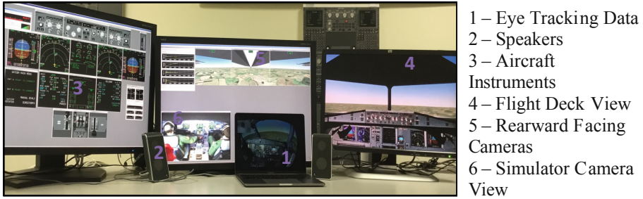
Fig. 1. Thales De-Brief Facility, in Voyager configuration, in addition to eye tracking data.
