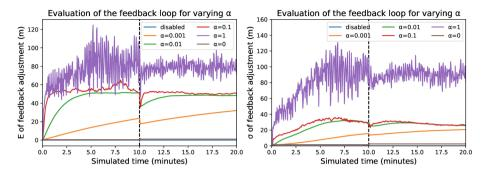
Fig. 4. Evaluation of the backoff parameter. Values are averaged along all values of u and  $\rho$ . Not considering new values ( $\alpha = 0$ ) has a similar effect to disabling feedback entirely. Plugging the feedback directly, without filtering, makes the system oscillate. Other values show how  $\alpha$  tunes the trade-off between reactivity and stability, with  $\alpha = 0.01$  both smooth and with an impact on the system comparable to  $\alpha = 0.1$
