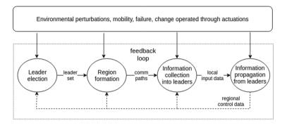
Fig. 2. SCR from a dynamical perspective—see description in Sect. 3.2. Notation: solid arrows represent required inputs or unavoidable perturbations; dashed lines denote possible feedback loops
