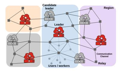
**Fig. 1.** SCR from a structural perspective—see description in Sect. 3.1. Notation: "gateway-like" nodes denote candidate leaders (red for active ones, grey for unelected ones); small grey squares denote relays; small grey circles denote users/workers (Color figure online)
