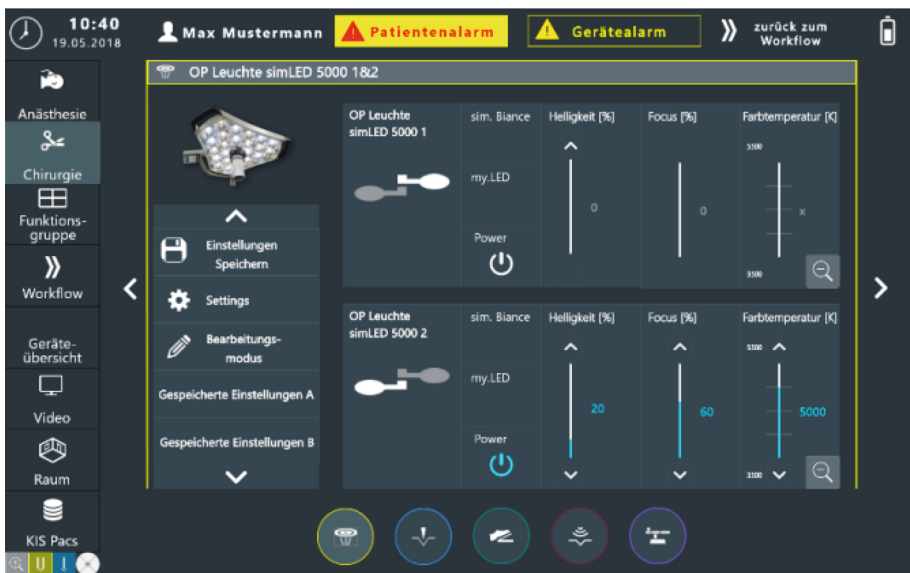
Fig. 2. GUI concept for the tablet control
