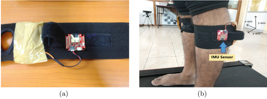
Fig. 1. (a) A closer look at Sparkfun 9DoF Razor IMU sensor. (b) Placement of the two IMU sensors around the shank of both legs of the candidate walking on the treadmill.
