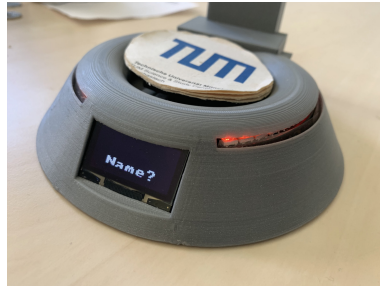
Fig. 7. Interaction methods in the form of LED stripes and a display
