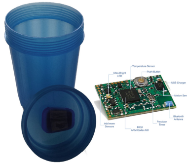
Fig. 2. Prototype 1: Cup with Development Platform MetaWear CPRO [25] and an accelerometer
