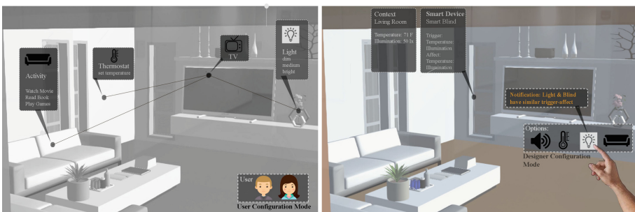
Fig. 8. Left: User Configuration Mode—Customize configuration of ambient environment to accommodate user’s personal preference. Use of data model for configuration of SBE. Right: Designer Configuration Mode—Explore combinations of smart objects and resolve conflicts.
