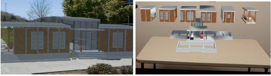
Fig. 9. Left: Preview mode: visualizing design in outdoors. Right: Architectural design mode: visualizing design and module library in MR environment.
