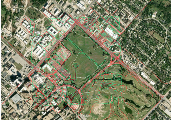
Fig. 4. Civil 3D drawing with imported InfraWorks model with aerial map and existing transportation surface.
