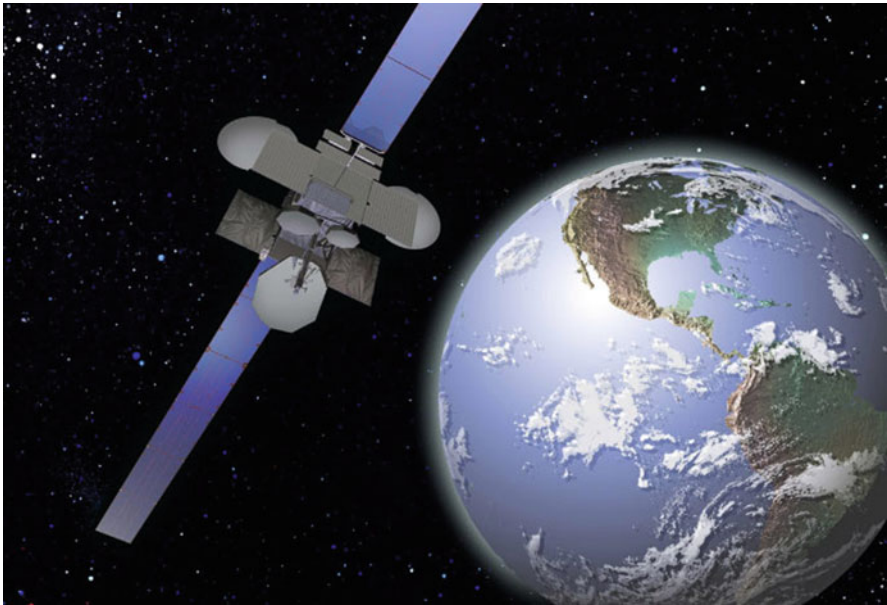
Fig. 4 The ViaSat-2 satellite can transmit at a rate of 160 gigabits/s (or the equivalent of 10,000 times the capacity of the Early Bird Satellite of 1965), and its lifetime is 10 times longer (Graphic courtesy of ViaSat)
