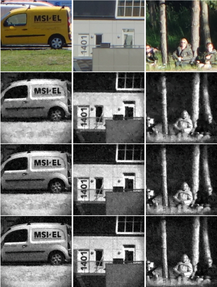
Fig. 7. Varying subsampling ratios - first row: visual image, second row: 5%, third row: 10% and fourth row 15% - to reconstruct sample images captured by the SPC.
