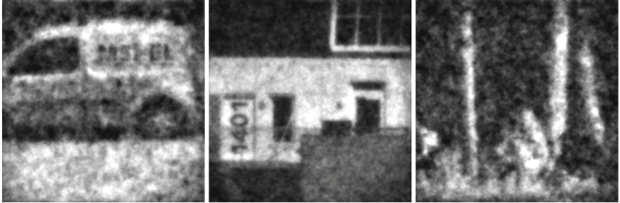
Fig. 6. Varying minimum subsampling ratios (2%, 3% and 3%) to reconstruct sample images captured by the SPC.
