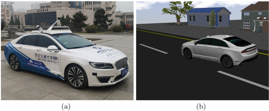
Fig. 4. (a) The self-driving experimental platform “Pioneer”, based on 2017 Lincoln MKZ hybrid model. (b) The simulation platform based on Gazebo. Various experimental scenarios can be built in this simulation platform.
