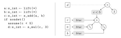
Fig. 3. The transformed program builds term trees that represent symbolic values. The boxes correspond to symbolic variables while the circles are the concrete representation of terms. Question marks denote unconstrained nullary symbols. Gray boxes represent path condition constraints.
