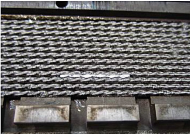
Fig. 10.18 Tin leakage at turn 3 of the inner winding of one module
