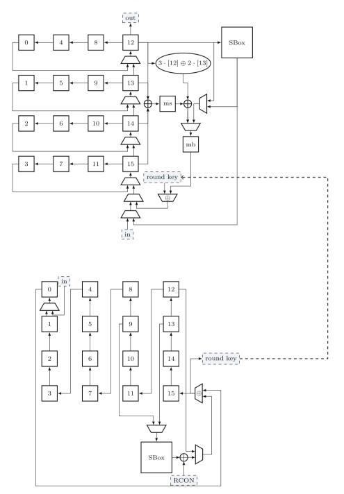
Fig. 2. (a) (upper part) The state. All datapaths depicted are 8-bit wide. The S-Box can be implemented as a shared module. (b) (lower part) The **keystate**. All datapaths depicted are 8-bit wide. The S-Box can be implemented as a shared module.
