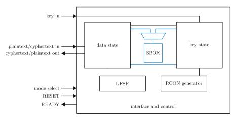
Fig. 1. High level view of the proposed architecture. The control module encapsulates the two state modules and some smaller utility modules. The public interface is described in Subsect. 4.1. The S-Box can be implemented either as a shared module or with a distinct copy for each state.
