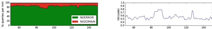
Fig. 1. Two anomalies in the ratio between DNS queries for valid and non-existent domain names over time (left), viewed in terms of entropy (right). Transforming the distribution to an entropy time series allows automated detection with standard anomaly detection techniques.
