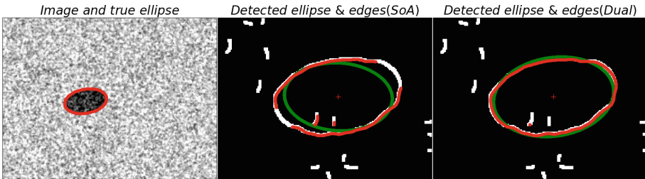
Fig. 3. A sample test image (left), the results of the SoA algorithm (middle), and of our method (right). The detected ellipse is drawn in green and the selected edge points are drawn in red. (Color figure online)
