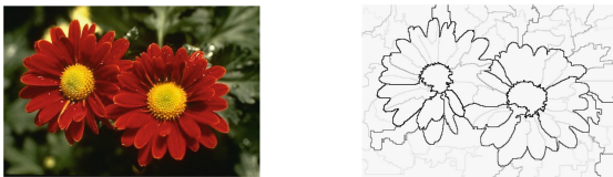
Fig. 2. Example of obtained result by a hierarchical image segmentation method: (left) original image; and (right) Ultrametric Contour Map (UCM).
