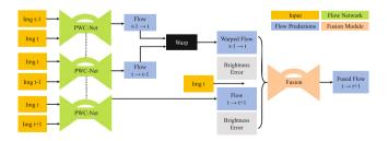
Fig. 1. Architecture of the proposed fusion approach.
