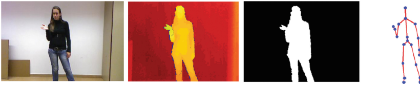
Fig. 6. The different raw visual modalities provided by the organizers of the ChaLearn challenge on Montalbano dataset. Neverova et al. [15] propose to focus on right and left hands, skeleton and audio.
