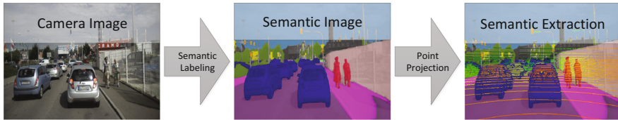
Fig. 5. Overview of the Autolabeling process for large-scale automated training data generation. Each pixel of the reference camera image is classified via an image-based semantic labeling network. Subsequently, the point cloud is projected into the camera image and the reference labels are transferred to the corresponding LiDAR points.
