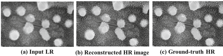
Fig. 5. An example of the reconstructed high-resolution image (magnification of \times 2.5 ): (a) Low-resolution image, (b) reconstructed output based on SRCNN scheme and (c) original test image.
