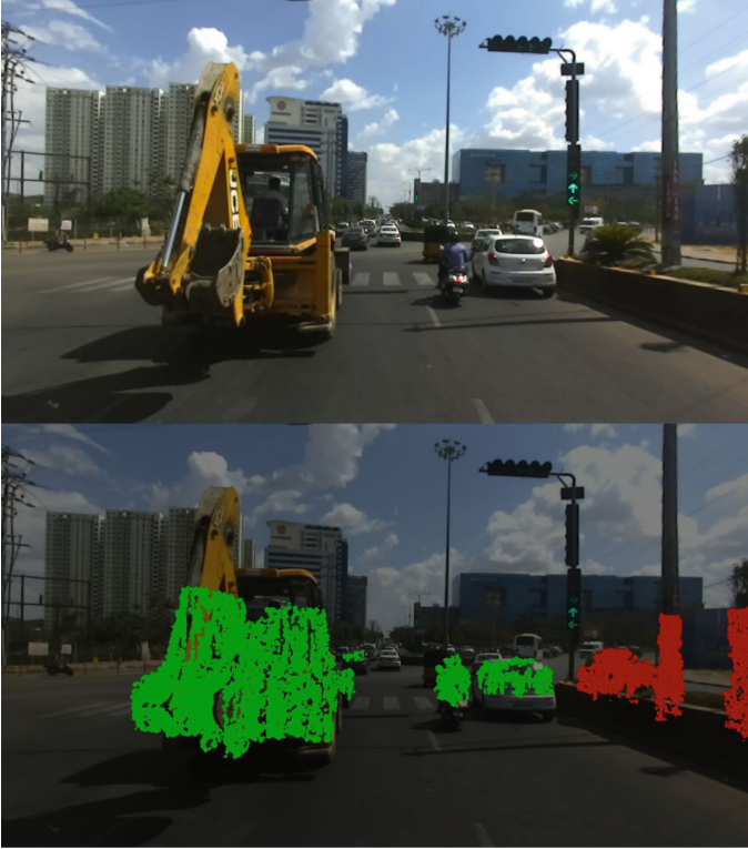
Fig. 1. (Top) Input stereo sequence, (Bottom) output of our motion segmentation green represents moving/dynamic and red represents static objects (Color figure online)
