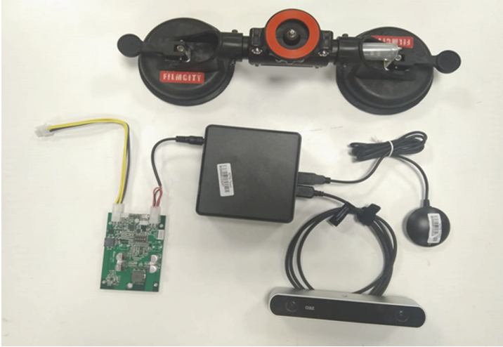
Fig. 4. An example of low cost data collection hardware kit built using the framework. From top left to right: a suction mount, DC voltage regulator, low cost compute, GPS and stereo camera
