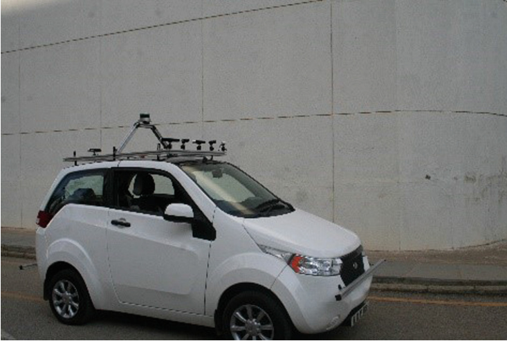
Fig. 5. An electric car mounted with stereo cameras, LIDAR, GPS and IMU
