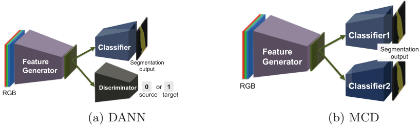
Fig. 2. Example of network architectures for domain adaptation [(a) domain adversarial neural network (DANN) [15] and (b) maximum classifier discrepancy (MCD) [30]]. When inputs belong to source samples which have labels, we train a feature generator and a classifier using the labels. When inputs belong to target samples which have no labels, we train a feature generator and (one discriminator in the case DANN is used or two classifiers in the case MCD is used) in an adversarial manner.
