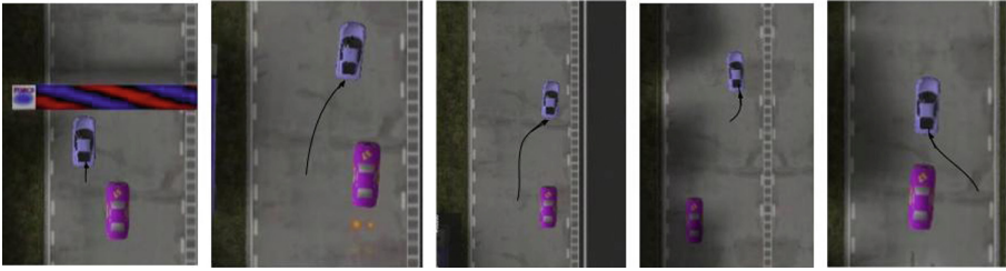
Fig. 4. Results of blocking behavior, in first three images, the purple car moves towards right to overtake our (blue) agent, our agent also moves towards the right to prevent the overtaking. In last two frames, the purple car is translating towards left and back to center and our car, also translates in center to block it from overtaking. (Color figure online)
