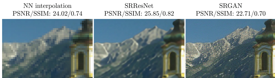
Fig. 1. Inconsistency between PSNR/SSIM values and perceptual quality.
