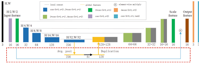
Fig. 5. U-net architecture for image enhancement proposed by Mt.Phoenix.
