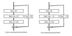
Fig. 5. We extend the original down-sampling residual architecture (left) to an upsampling version (right). We use a  $1 \times 1$  fractionally-strided convolution as a shortcut and adopt reflectance padding.
