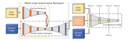
Fig. 2. An overview of MSG-Net, Multi-style Generative Network. The transformation network explicitly matches the features statistics of the style targets captured by a Siamese network using the proposed CoMatch Layer (introduced in Sect. 3). A pre-trained loss network provides the supervision of MSG-Net learning by minimizing the content and style differences with the targets as discussed in Sect. 4.2.
