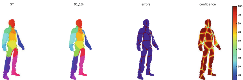
Fig. 5. Confidence in the segmentation. From left to right, the ground truth segmentation (GT), the result of the CNN segmentation, the error image (blue for correct, red for error in the segmentation) and the confidence image computed as a probability using the softmax function and expressed in percentage. (Color figure online)
