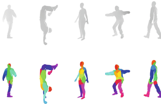
Fig. 3. Examples of simulated synthetic range images (top row) with their corresponding segmentation into 33 body parts (bottom row). Each color correspond to a distinct body part. Note the presence of occlusions (for instance the self-occlusion of the left leg in the first column or the disconnected leg and head in the second column).
