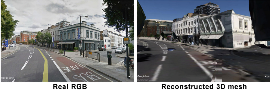
Fig. 4. A sample of RGB vs reconstructed 3D meshes (used for training) from the same location. Note the significant geometric, texture and illumination inconsistencies introduced by the reconstruction in contrast to a real-world capture. The darker regions in the right and left are tree meshes. While these meshes are very difficult to use for learning something at the ground level, from a birds’s eye viewpoint they look similar to the real RGB image. (Color figure online)
