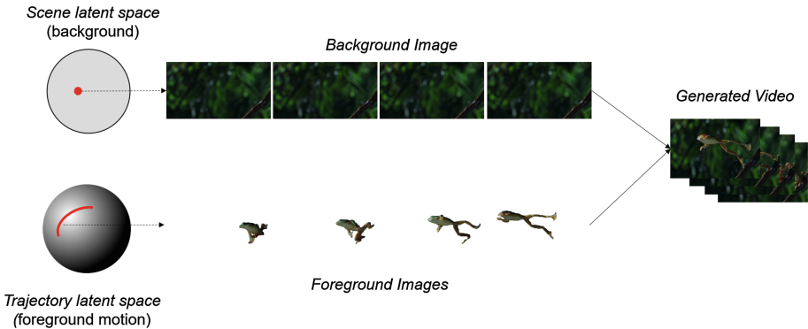
Fig. 1. Video Generation in VOS-GAN: we employ a scene latent space to generate background and a foreground latent space to generate object appearance and motion.
