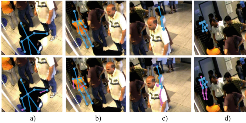
Fig. 7. Examples of predictions on Salsa. Top row: OpenPose results (in blue). Bottom row: missing joints predicted by our method (in magenta). (Color figure online)
