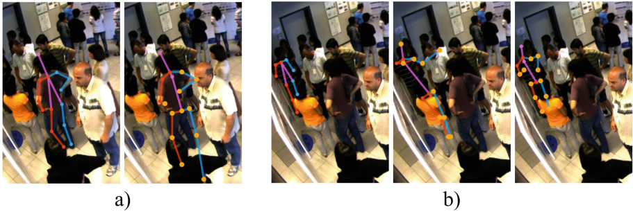
Fig. 4. Comparison between OpenPose and Regional Multi-Person Pose Estimation (RMPE) [10]. (a) and (b) left show OpenPose predictions, while (a) right and (b) center, right show RMPE predictions. Orange joints have a confidence score below 0.2. (Color figure online)
