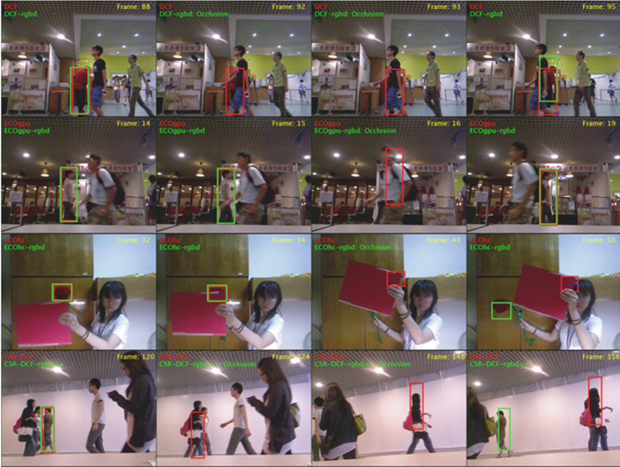
Fig. 4. Short-term and long-term occlusion examples comparing the original methods (red) and their RGBD versions (green). Top row – DCF, second row – ECOgpu, third row – ECOhc, bottom row – CSR-DCF. (Color figure online)
