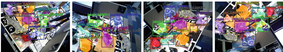
Fig. 13. Results of Mask-RCNN [19] trained on synthetic images only with the feature extractor frozen. The images were taken with the AsusXtionPROLive camera in a highly cluttered environment under various poses.
