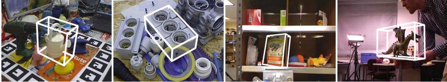
Fig. 1. Estimation of 6D pose, i.e. 3D translation and 3D rotation, of a specific rigid object. This task is considered in the BOP benchmark [25].
