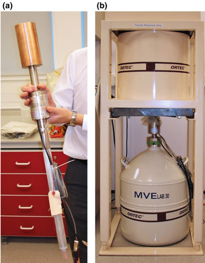
Fig. 3.1 a Example of a HPGe gamma detector showing the detector head, the cartridge containing electronic management system and the dip-stick which is immersed in liquid nitrogen to cool down the detector to 77 K; b the detector encased in a lead shield with the dip stick immersed in a liquid nitrogen tank. NB: The liquid nitrogen tank should be filled on a regular basis (every 7–10 days) to maintain a fully operational detector
