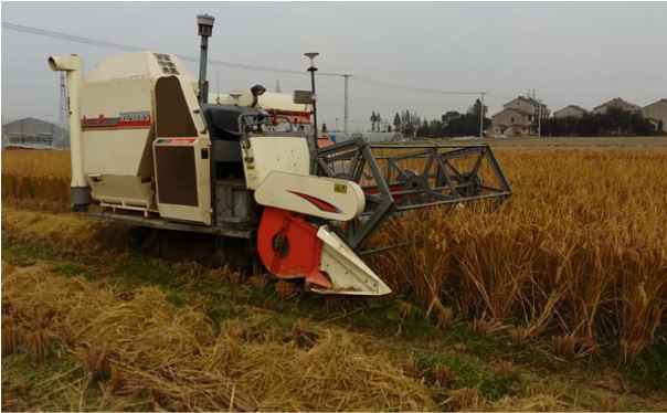
Fig. 6. The prototype of automated guided combine
