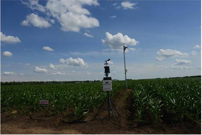
Fig. 1. Environmental data acquisition equipment installed at the experiment site
