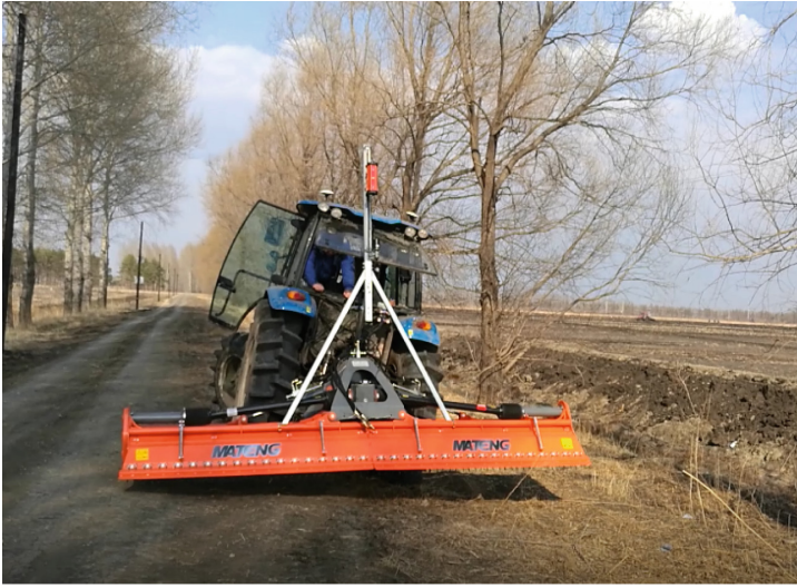
Fig. 6. The self—balancing adjustment of the graders
