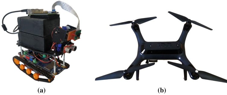
Fig. 6. The used robots: (a) the small-scale rover, (b) the small-scale UAV.
