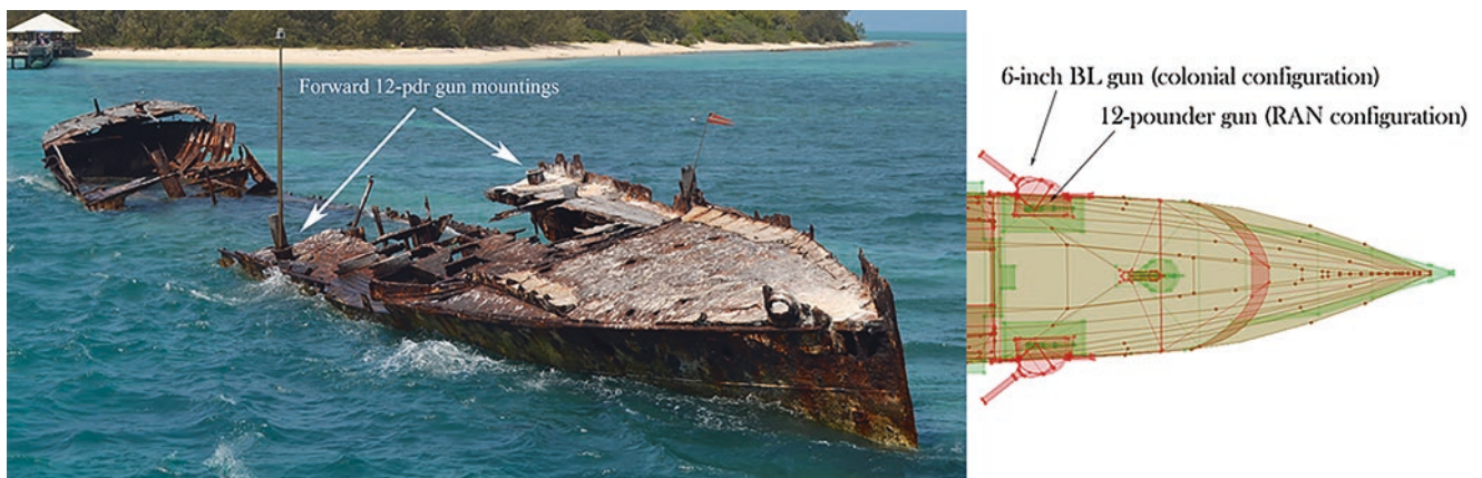
Fig. 6.6 Left: Protector's surviving hull, showing the locations of its forward 12-pounder gun mountings; right: superimposed digital models of the vessel's colonial and national navy configurations reveal the posi-
