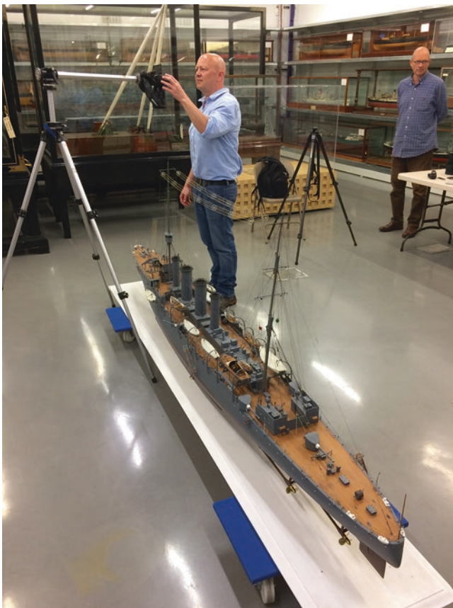
Fig. 12.3 Photogrammetric survey of the builder's model of HMS Falmouth , carried out by Historic England Geospatial Imaging team at the Chatham store of the Imperial War Museums. Antony Firth, Fjodr
