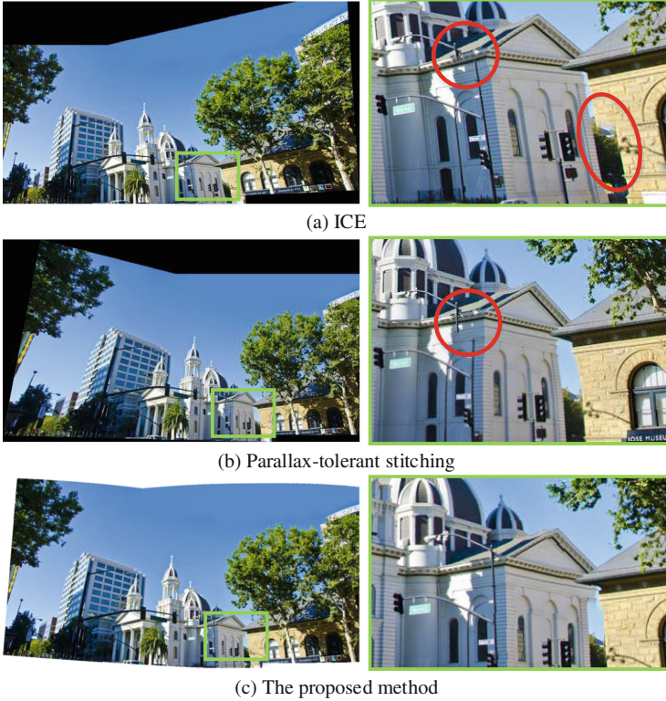
Fig. 7. Comparison with seam-assist stitching methods, i.e. (a) ICE, (b) parallax-tolerant stitching [29] and (c) the proposed method. For comparison, we highlight some details in the green boxes. Errors are highlighted in red circles. (Color figure online)
