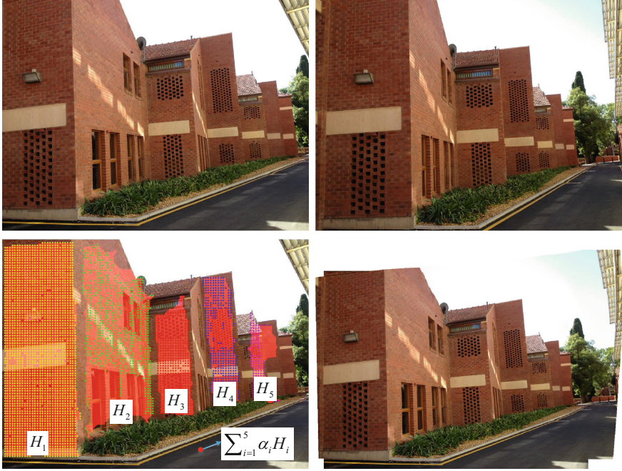
Fig. 1. An illustration of our method. The top row display two input images taken casually and the scene contains multiple distinct planes. The bottom row shows the detected planes and transition regions (left) and the final stitching result (right). Planar regions are warped by planar homography \mathbf{H}_i , and the transition regions are transformed by the local weighted homography \sum_{i=1}^5 \alpha_i \mathbf{H}_i .
