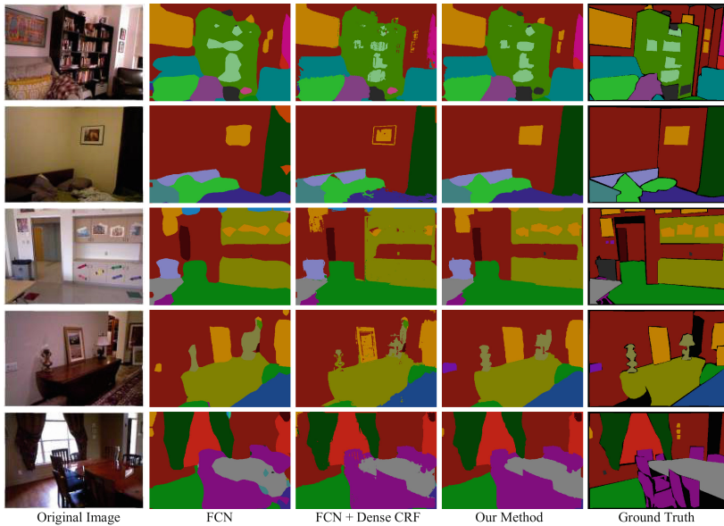
Fig. 5. Qualitative comparison with the other approaches. Left to right column: Original Image, FCN [15], FCN+ Dense CRF [13], Our Method and Ground Truth. Different colors indicate different classes.
